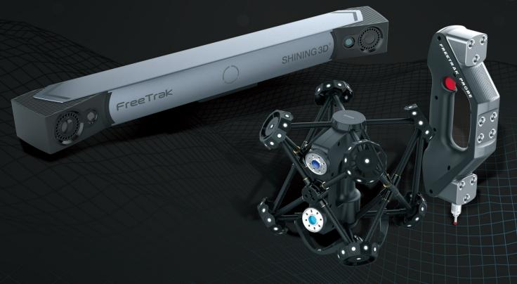
Portable Wireless Optical Coordinate Measuring System:
